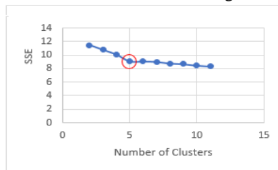
Fig. 3. Elbow Method; SSE vs Number of Clusters
